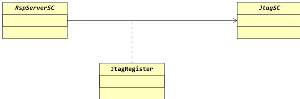
Figure 7: Top level class diagram for a unified RSP to SystemC JTAG interface.
